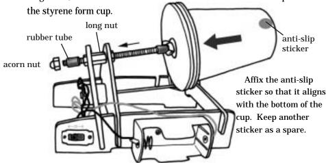
Hang the large (and thin) rubber band around the pulley and the shaft of the motor. Put the battery in the battery box and turn the switch to the left and check if the cylinder moves to the direction of the arrow (left).
