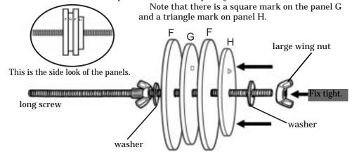
Insert the long screw into the pipe 2 and a washer. Then attach the styrene form cup and another washer. Fasten them with a large wing nut. This makes the cylinder unit.
