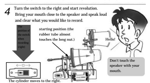
When you finish recording, turn the switch back to the center and stop the motor. (The phonograph can record about 15 seconds maximum.)
