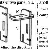
Put the pipe 3 into the panel K. Then insert another panel K into the lower cuts of two panel N's
