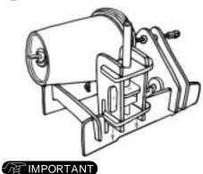
Put the post into the cuts of the body completely. 12
