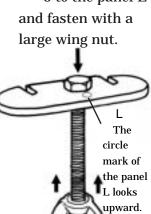
Attach the bolt 24 Put two panel M's 25 Fasten 16 to 24 with the into the panel L.
