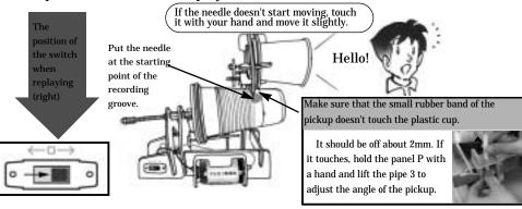
When you finish recording, turn the switch back to the center and stop the motor. (You can replay as many as you like by the same step. But you can't record on the same cup you once used.) Remove the battery and put the needle cover after using.
