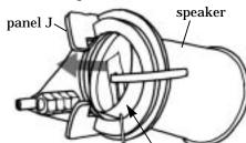
Push the cup in completely. Do not mind the distortion of the cup where it touches the panel I.
