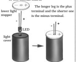
Bend the legs of the LED to right and left. Cover with the upper light stopper as the plus terminal comes to the plus mark and the minus terminal to the minus mark. Fasten with a piece of a Scotch tape as shown in the figure.
