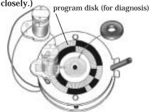
Align the start line of the program disk (for diagnosis) with the line of the light holder.
