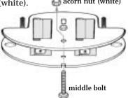
Now the drive unit is completed. Turn it upside down to be the right position. Two tires and the plastic acorn nut support this unit.
