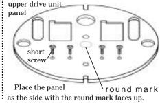
Fit the driving motor units (right and left) in the holes of the upper drive unit panel upside down. (Pay attention not to mistake right and left of the driving
