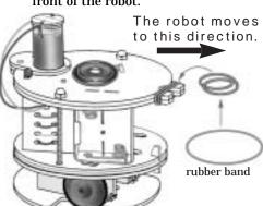
Put the felt-tip pen through upper and lower bodies from the rubber band to the ground.
