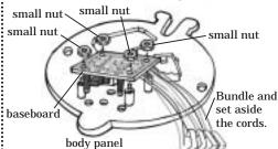
Fit the projecting parts of the base board (light-emitting diodes and optical sensors) into the holes of the body panel.
