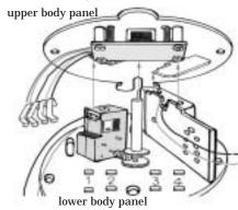
Fasten the lower body panel and the upper body panel with large bolts and large acorn nuts.
