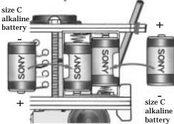
Be sure to use unused batteries. (Alkaline batteries are desirable.) The switch is behind the baseboard. The switch is turned on when moved to the right and turned off when moved to the left.
