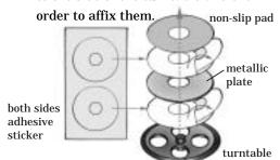
The hole at the center of the turntable faces down.
