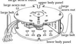
Screw acorn nuts with hands completely without using any tools.
