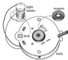
Put the program disk (for diagnosis) on the shaft of the turntable and fasten with the magnet. Then set the light holder. (Set it firmly and
