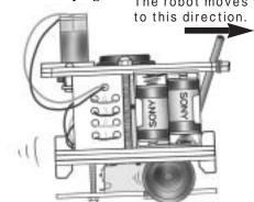
The robot moves drawing a trace on the paper turning on the red light of the LED in the direction of a turn. (When it goes straight, both lights are turned on and when stops, turned off.)
