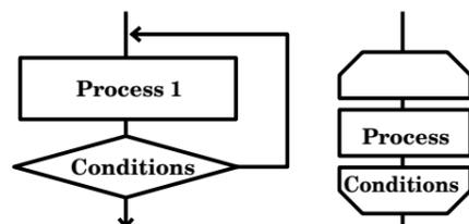
Depending on the conditions, the flow returns to a previous process. The flow proceeds to the following process once certain conditions have been fulfilled.
