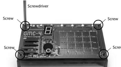
\* Be careful not to damage the circuit with the screwdriver.
