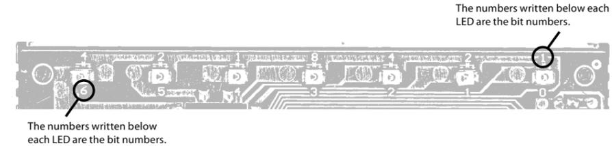
The binary LEDs are used to display "binary numbers." Numbers are given for binary LEDs 0 through 6, and these numbers are referred to as bit numbers. If an LED is lit up, then that LED is displaying a "1," and if an LED is off, then that LED is displaying a "0." Repeatedly pressing the INCR key changes the binary LED display in the order given below.
