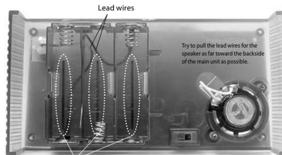
Pass the black and red lead wires around the protrusions in the three rows on the main unit.
