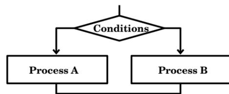
The diamond shape indicates the branch instruction. Process is divided into branches in accordance with certain conditions. However, no matter how much a process is divided up, the flow must always return to one place. By setting up one start and one end for each process, you can make it difficult for malfunctions to occur, even for complex programs. Incidentally, branches are managed using markers called execution flags that demonstrate the results of the command.
