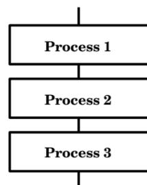
Process 1, Process 2, and Process 3 are executed in sequential order.
