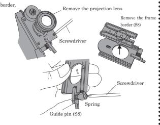
Remove only the spring from the S8 guide pin. Attach the removed spring to the W8 guide pin. Attach the W8 guide pin to the frame border with the screw.
