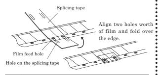
4 Setting 8mm Film (Double) \* A screwdriver is required.
