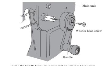
Install the handle to the main unit with the washer head screw.
