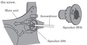
**2** Remove the frame border and replace the S8 guide pin with the W8 guide pin.
